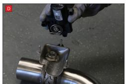
now be able to see the torsion spring (This must stay on the electronic valve motor to work with Scorpion Exhaust).
